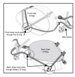
Make sure the front compression strap and back mounting strap pass through the correct D rings as shown above to ensure a proper fit. The back strap has to pass through 2 D-rings.
