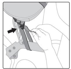
Loop front strap around frame or secure point thread through buckle and pull until tight. Secure all loose end and keep away from moving or hot parts. Use of a heat shield of muffler guard may be necessary.
