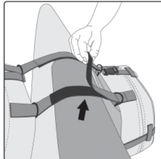
Place hook and loop webbing over seat and level bags. Adjust height of both bags and attach webbing together. Take caution that bag is not on hot or moving parts.
